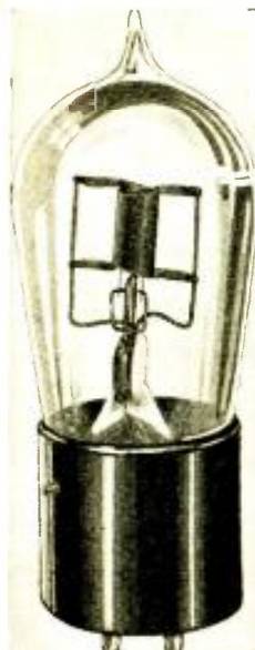
Fig. A The "K" tube, designed especially for relay work.
